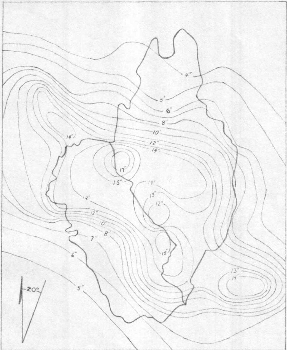
Figure 13. Transposition of Storm MR 6-15 over the Skunk River Basin above the Squaw Creek junction
