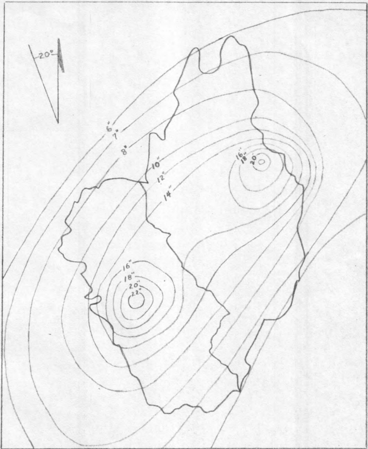
Figure 9. Transposition of Storm MR 4-24 over the Skunk River Basin above the Squaw Creek junction
